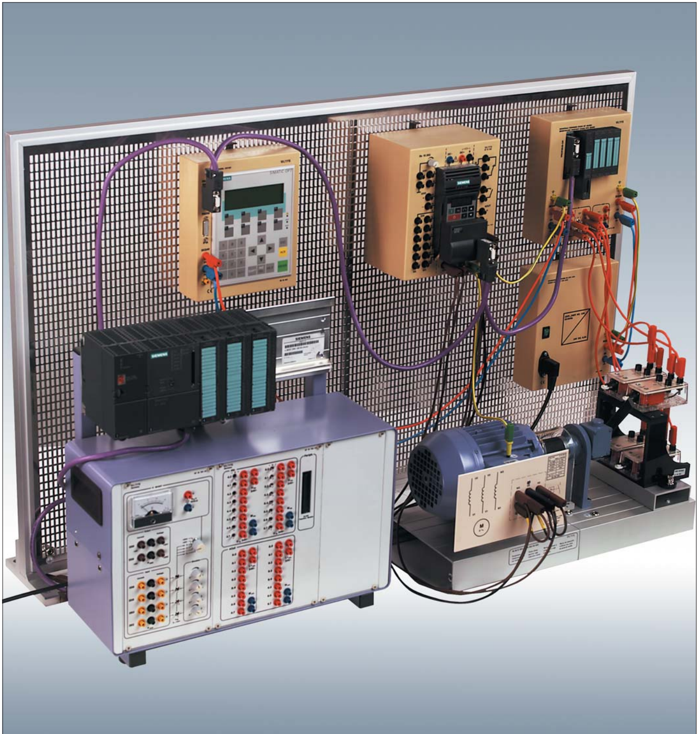
Power train with PLC, frequency inverter, I/O group and operator panel – interconnected via Profibus DP. Please ask for our catalogues on power electronics/drive engineering and on automation.
