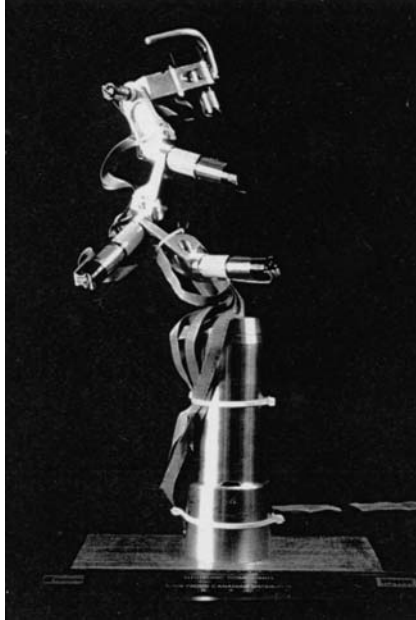
FIGURE 4.31. DIESTRO, a six-axis isotropic manipulator.
