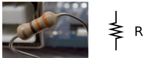
Fig. 7.1: Resistor (Ohms): resists the current flow, V = iR (think of a narrowing in a pipe (a) Element (b) Resistor circuit diagram.
