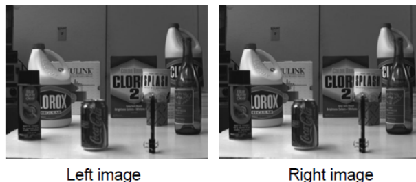
Fig. 9.8: Seeing in three dimensions with a pair of calibrated cameras: building a disparity (depth) map.
