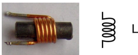
Fig. 7.3: Inductor (Henrys): stores energy in a magnetic field, V = L \frac{di}{dt} (think of a flywheel in the pipe.) (a) Element (b) Inductor circuit diagram.
