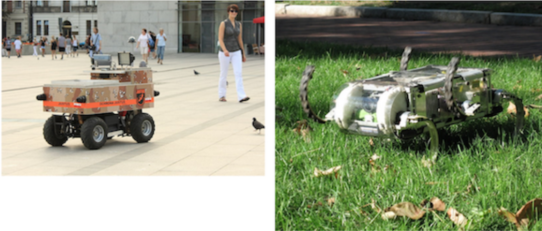
Fig. 1.8: Mobility in simple and complex domains. a) Justus security robot in front of Krakow railway station [MP18]. b) Rhex: DARPA project on compliant six legged robots. [Wik18e]
