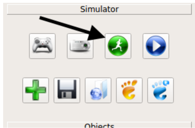
Fig. 22.18: The time warp button; press it multiple times to cycle through 2x, 3x, and 0.5x speeds
