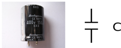
Fig. 7.2: Capacitor (Farads): stores energy in an electrical field, i = C \frac{dV}{dt} (think of a storage tank). (a) Element (b) Capacitor circuit diagram.
