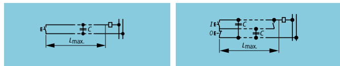
Figure 55: Two-wire control (left) and three-wire (pulsed) control
