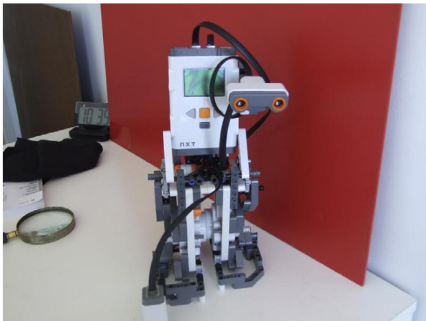
FIGURE 40.1 This humanoid robot has an ultrasonic sensor (looking like a pair of eyes, see also Figure 32.6) aimed straight ahead, so that the robot can detect an obstacle in its path before the robot collides with it.
