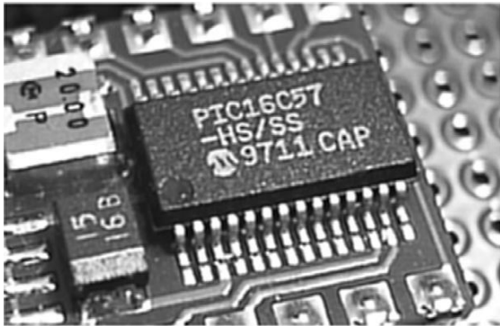
FIGURE 37.4 This member of the PIC family of controllers is in a surface-mount package that has 28 pins spaced 1.27 mm apart. Twenty of the pins are for input/output. In addition to the units shown in Figure 37.3, the chip carries two digital timers, an 8-bit real time clock, and a watchdog timer. It runs on a 2.5 V to 6.25 V supply, at up to 20 MHz.
