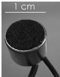
FIGURE 26.7 An electret microphone ‘insert’ usually has a built-in FET amplifier to provide the first stage of amplification.
