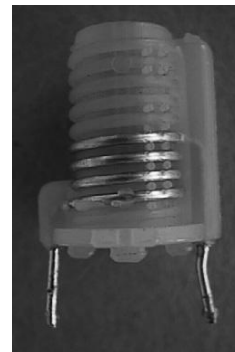
FIGURE 7.4 This VHF tuning coil with 3.5 turns of wire has a self inductance of 0.114 \mu\text{H} .
