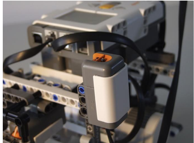
FIGURE 40.5 This robot has an upwardly-directed light sensor, which is used to detect shadows falling on the robot. It is used to give the robot the behaviour of a housefly. If the light falling on the fly is more-or-less constant, it ignores the small changes. But if there is a sudden fall in light intensity, the robot dashes away at high speed. It is responding in the same way as a housefly, ignoring small changes in light intensity but, when you try to swat it with your hand, responds to the sudden fall in light intensity as your hand nears the sensor.
