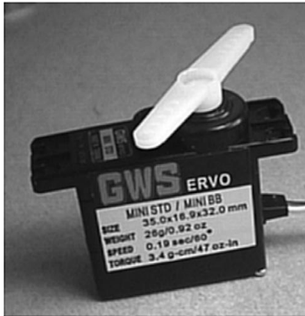
FIGURE 33.7 A small servomotor of the kind used in flying model aircraft and robots. The ‘horns’ (white levers) are used for connecting the motor to the mechanisms that it drives.
