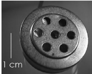
FIGURE 26.6 A crystal microphone ‘insert’, intended for installing inside a protective case. The crystal is shielded from stray magnetic fields by an aluminium screen. This should be connected to the 0 V line of the amplifier.
