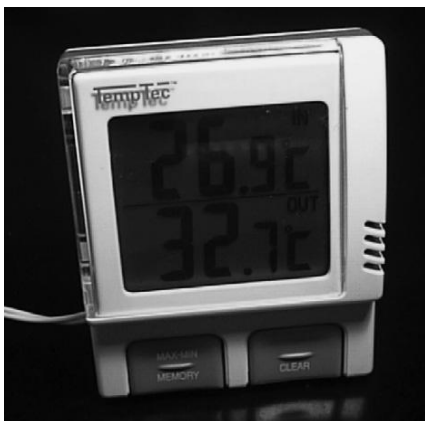
FIGURE 23.11 An indoor/outdoor thermometer uses an LCD to display the temperature at two sites. It runs for months, day and night, on a single 1.5 V AAA dry cell.
