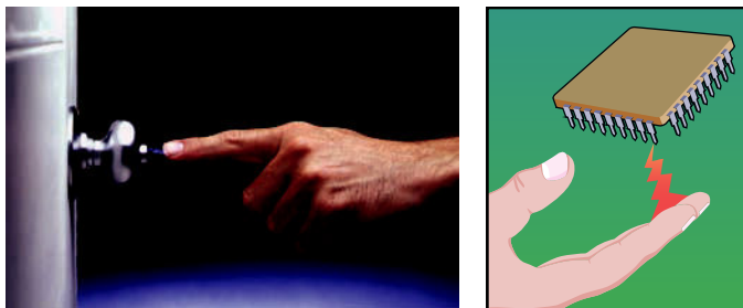
Figure 9-47 Electrostatic discharge (ESD). Photo courtesy RTP Company, www.rtpcompany.com .
