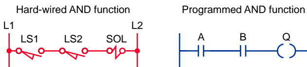
Figure 9-54 Hard-wired circuit and the equivalent PLC logic program for an AND logic control function.
