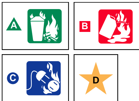
Figure 1-14 Types of fire extinguishers and their applications.
